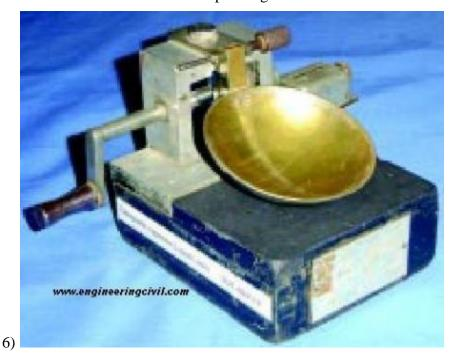
**Procedure to Determine The Liquid Limit of Soil**
